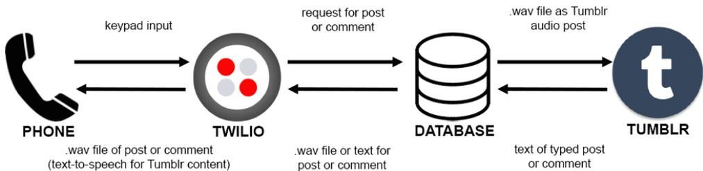
**Figure 1. Design of xPress, an IVR system that supports audio-based blogging through a landline or cell phone.**
